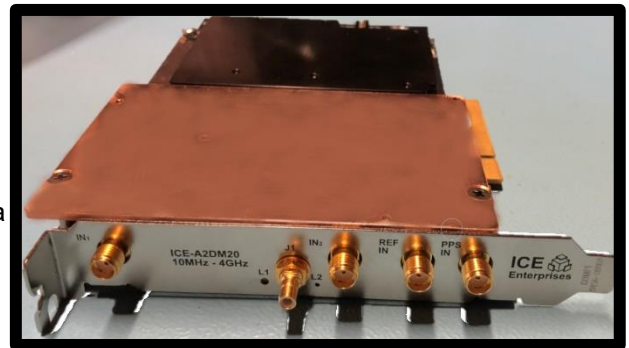
Figure 1 ICE-A2D-m20 on a PCIe 8-Lane, PIC8S(Short)
