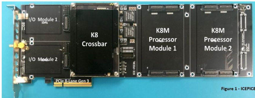
Figure 10 - ICEPIC8 showing I/O module sites, K8 Crossbar, and Processor Module sites
